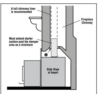
A non-combustible seal is required at the damper area (to prevent dilution air from entering the chimney). See Direct Connect Positive Flue Connection on this page. A seal-off plate method is shown here.
