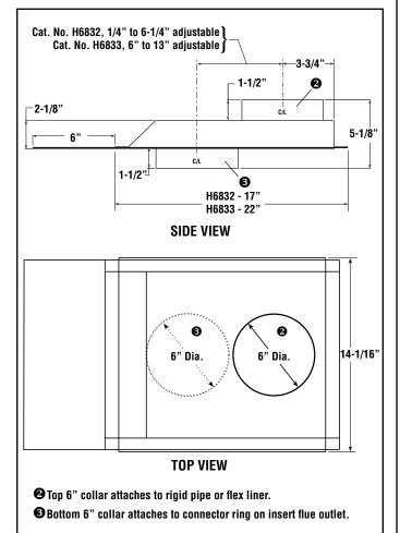
Figure 9 - Offset Box Dimensions
