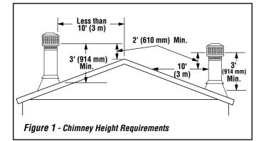
To pass inspection in nearly any jurisdiction, the chimney must meet both safety and exhaust flow requirements. The (3' by) 2' by 10' rule applies to both masonry and factory-built chimneys.
